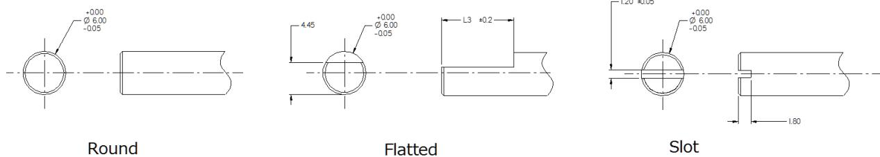
Note: For flattened shaft, L3 should be defined as "FMS=20mm, L3=8.7mm, FMS=25, L3=13mm"
